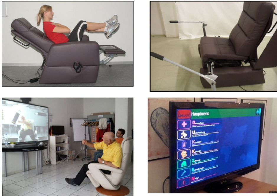
Fig. 8. The GEWOS chair (top left), in row training/gaming modus (top right), gesture gaming/exercising (bottom left), menu for the ambient-assisted support controlled by the chair (bottom right) [23].
