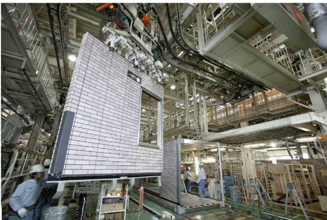
Fig. 5. The concept of Robotic Industrialization applied by the company Sekisui Heim to industrially personalize buildings on the assembly line (Image: courtesy of Sekisui Heim).
