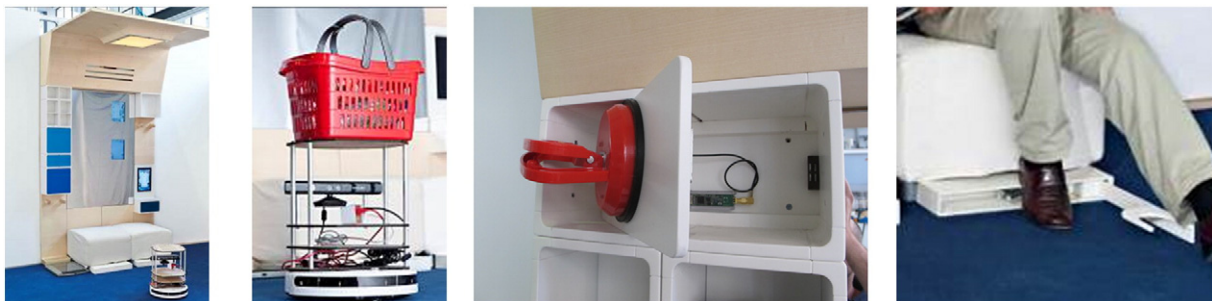
Fig. 9. Smart wall terminal prototype with functionality: mobile robot communicating with the wall, smart cabinets and assistance for dressing/undressing [30].
