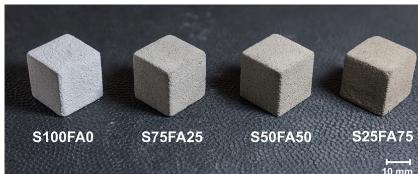
Fig. 6. Powder-based 3D printed green cubes using geopolymer powders with different slag/fly ash ratios. (For interpretation of the references to colour in this figure legend, the reader is referred to the web version of this article.)
